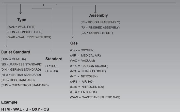
Outlet Standard: British Standard Type: Wall Type Standard: US Standard Gas: Oxygen Assembly: Complete Set
