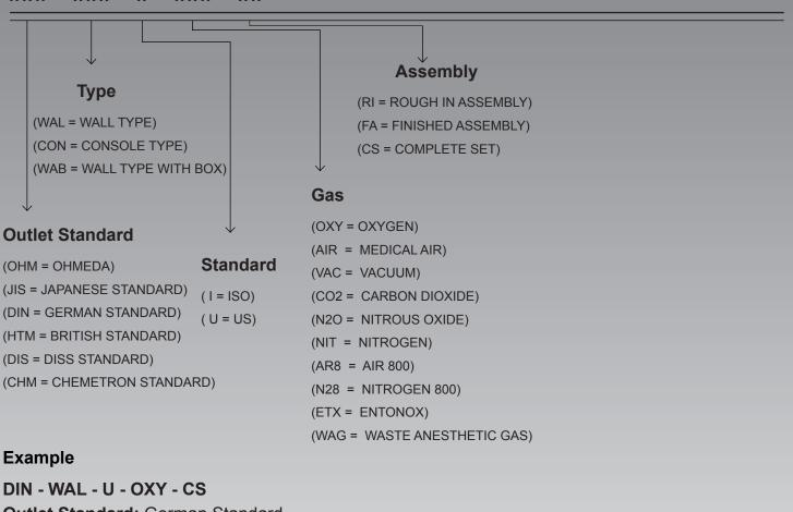
**DIN - WAL - U - OXY - CS Outlet Standard:** German Standard **Type:** Wall Type **Standard:** US Standard **Gas:** Oxygen **Assembly:** Complete Set
